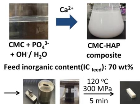
Fig. 2. Synthesis of the composites of CMC and HAP by coprecipitation.
